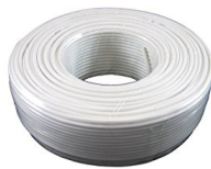
SCL-100FT-SJTW18/6 WHITE 100 FT. CORD, SJTW 18 AWG 6-CONDUCT ( WH/BK/GN/PU/GY + RED FOR EMERGENCY)
